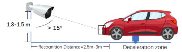
2. For Road Surveillance ( 30km/h< Speed < 70km/h )
