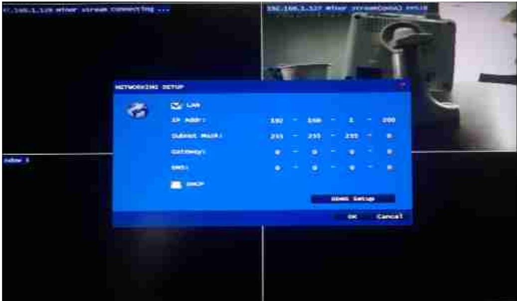
Present in the NVR applications, the default use of LAN (fix IP)-configured. When the NVR and IP Camera in the same LAN, only need to configure the IP address and subnet mask. Gateway and DNS is not required with the project.
