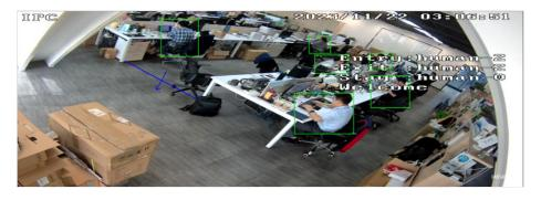
12MP fisheye can provide Omnidirectional(360°) view, and have several detection line crossing to cover the whole scene.
