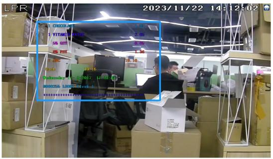
Video and the corresponding overlay POS information can be shown simultaneously in both live view and playback. With this system, user can search text to find out bills and the video recordings.
